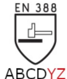
In 2016, ISO 13997 added 2 new letters to the standards logo: Y and Z. **Y** is for the new straight blade cut resistance methodology on a scale of A – F. The last digit **Z** is for impact protection. This classification is rated P, F or X. Therefore, an EN388 glove might have a marking example of 4-4-4-2-C-X
